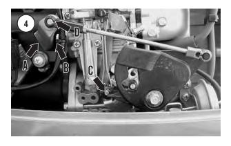
corded prior to removal. The screw should be approximately two turns out from the lightly seated position.
