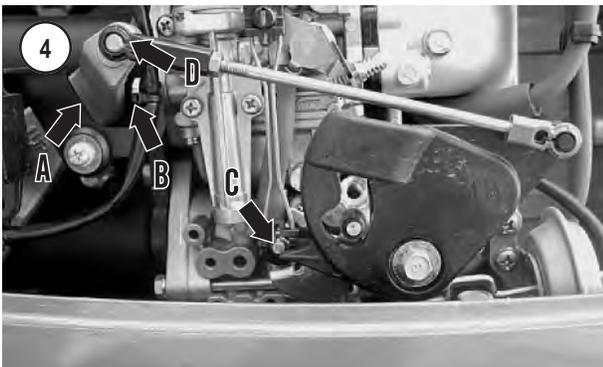
corded prior to removal. The screw should be approximately two turns out from the lightly seated position.
